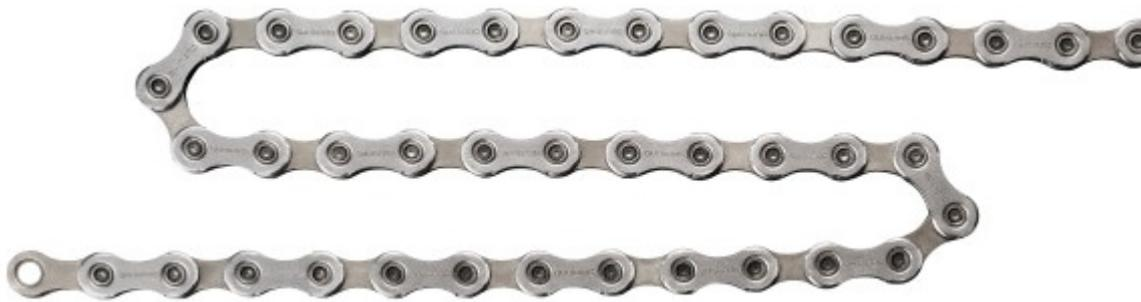
**Chain:** There is more to the new 105 level HG600 chain than just 11 speed compatibility. The chain has an asymmetric design with outboard plates designed specifically to aid front shifting, and inboard plates to improve rear shifting. It means that if you are taking the chain of the bike for cleaning, make sure you install it the same way! The outside has text engraved in the plates – the inside is blank!
